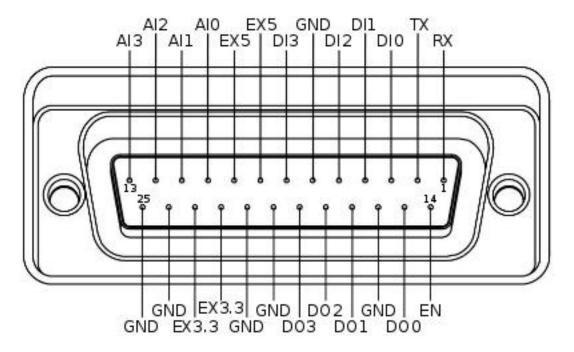
The minimum number of required pins for serial communication is three; TX, RX, and GND. Additionally EX3.3 or EX5 can be used for powering external devices, such as line transceiver.
